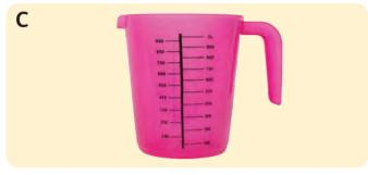
We can measure how much liquid we have by using A thermometer measures temperature and tells a measuring jug and looking carefully at the marked us how hot or cold it is. Temperature is measured units. This jug shows litres and millilitres.
