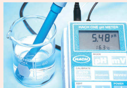
▲ Figure 7 A pH meter measures pH, often to one or more decimal places.
