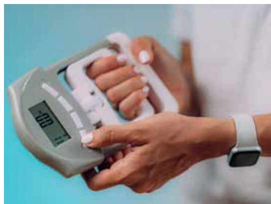
▲ Figure 27 A grip strength meter. You squeeze the meter as hard as you can for 5 seconds and record the reading.
