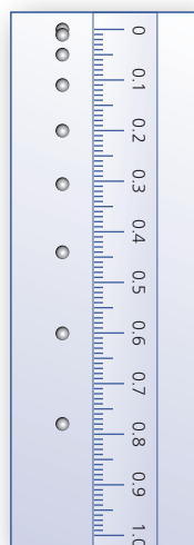
▲ Figure 2.7 Apparatus to determine the acceleration of free fall
