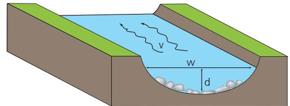
$w = \text{width}$     $v = \text{velocity}$     $d = \text{depth}$
