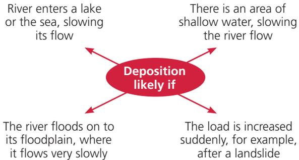
▲ **Figure 10** Conditions that are likely to result in deposition.
