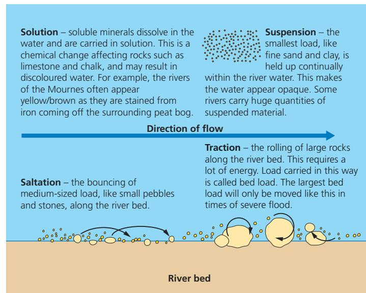
▲ **Figure 9** Methods that a river uses to move its load.
