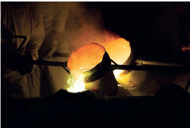
▲ Figure 1.1 In sand casting, molten metal is poured into a sand mould
