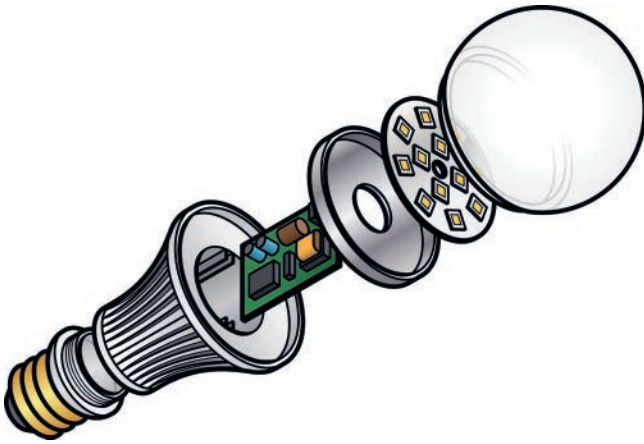
Figure 2.19 An exploded diagram of an LED (light emitting diode) lightbulb
