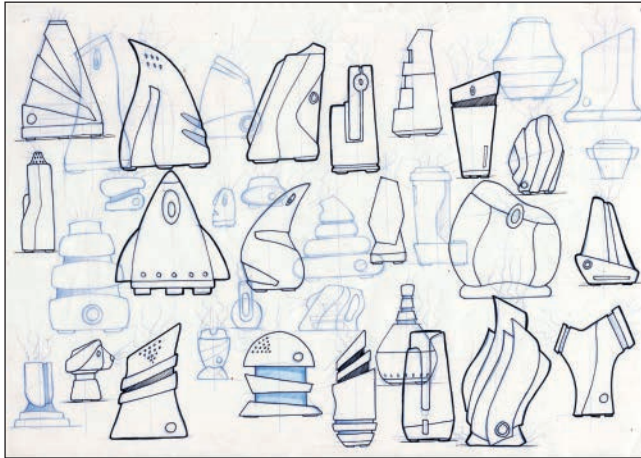
Figure 2.6 Thick and thin lines used to enhance 2D freehand thumbnail sketches
