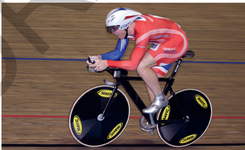
Figure 1.1.21 High-performance bicycle made from carbon fibre
