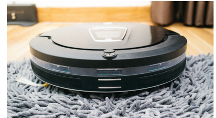
▲ Figure 1.2 Robotic vacuum cleaners use AI technology to map their environment, by using navigational sensors.
