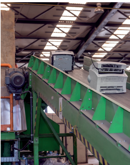
Figure 1.32 Used office printers ready to be disassembled inside a recycling plant.
