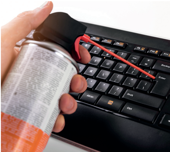
Figure 1.30 Using compressed air to clean a keyboard
