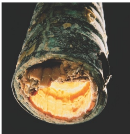
Figure 3.8 The effect of hard water on a heating pipe.
