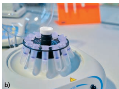
Figure 1.7 a) Homogenisation of potato cells using a mortar and pestle; b) spinning homogenate in a centrifuge; c) the separation of dense starch grains in a pellet from less-dense cytoplasm in the supernatant
