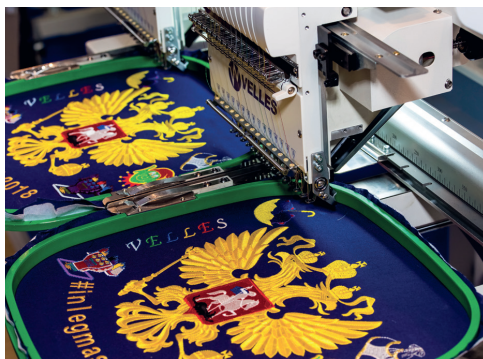
Figure 1.8 A CNC embroidery machine producing a multi-coloured logo
