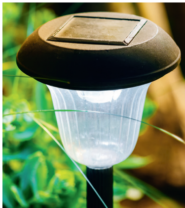
Figure 1.18 This solar-powered garden lamp recharges during the day.
