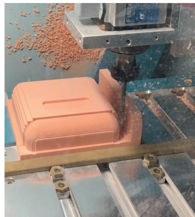
Figure 1.7 CNC router machining a prototype from polyurethane modelling foam
