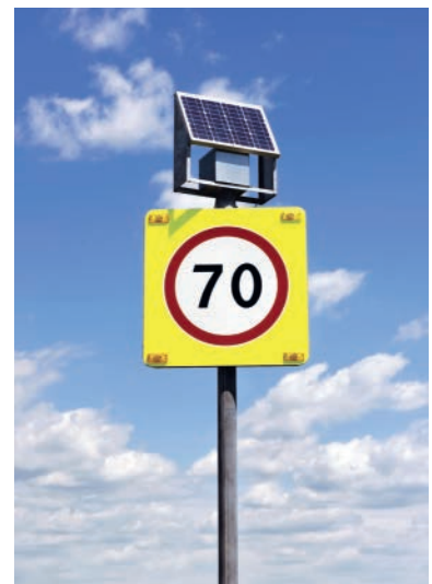
Figure 1.5 Electronic road sign powered by solar energy
