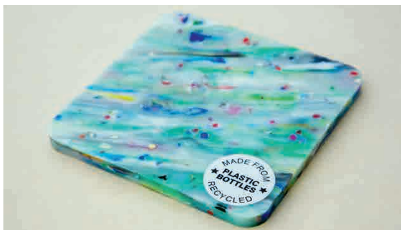
Figure 5.23 Drinks coaster made from recycled plastic (HDPE)
