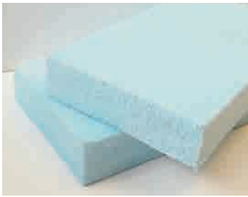
Figure 5.3 Styrofoam™ is strong, lightweight, water-resistant and a good heat insulator.
