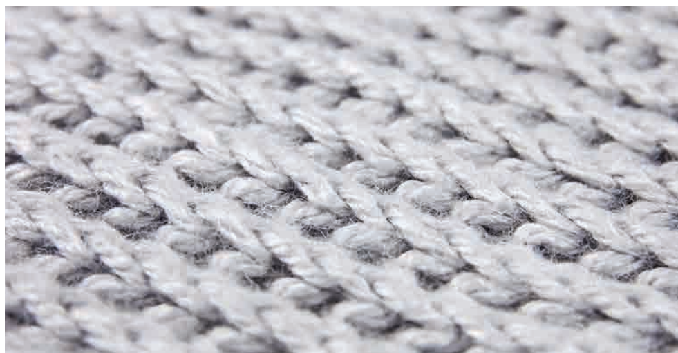
Figure 5.34 Knitted fabrics are made up of rows of interlocking stitches.
