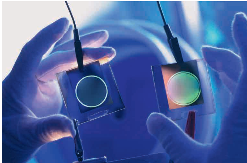
Figure 5.39 Conductive polymers are plastic products that can conduct electricity.
