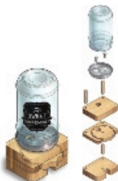
▲ An isometric and exploded view of a sweet dispenser
