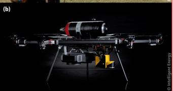
Commercial drone operators, such as those working in the inspection, mapping and cinematography sectors, are often limited by the flight time capabilities of battery-powered drones. The heavier the aircraft, the shorter the flight. Batteries require lengthy recharging times, increasing the time required to complete a job. Batteries can also be heavy, especially when increasing the power needed, thereby limiting any additional equipment that may be required.
