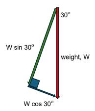
As the box is at rest, the total force parallel to the slope is zero, and so the frictional force acting up the slope is:
