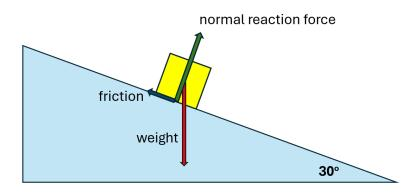
To find the frictional force, resolve the weight into two components parallel to and perpendicular to the slope.
