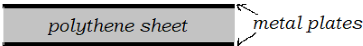
Figure 2: A 370-pF capacitor
