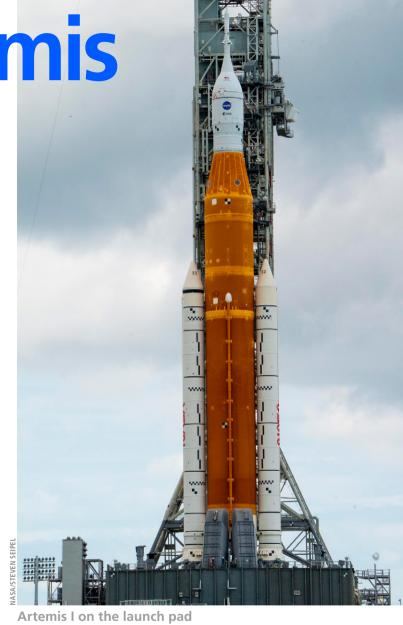
SLS is a super heavy-lift rocket capable of launching the *Orion* spacecraft with four astronauts and cargo directly to the Moon. It has about 40 MN of thrust, which is 15% more than the *Saturn V* rocket used for the Apollo missions. For comparison, the two engines of an Airbus A320–200 aircraft together can provide about 240 kN of thrust. The SLS has a top speed of 39 500 km/h, whereas *Saturn V* had a top speed of 28 000 km/h.
