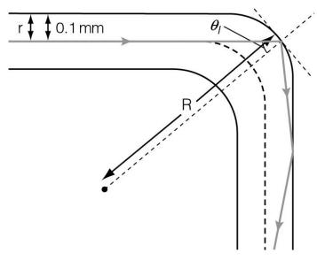
From the diagram,  $\sin \theta_i = R/(R+r)$  where r is the radius of the fibre = 0.2 mm / 2 = 0.1 mm
