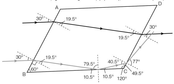
If, instead, the refracted beam hits *BC*, the angle of incidence will be  $90 - (180 - (60 + 90 + 19.5)) = 79.5^{\circ}$  (see diagram).
