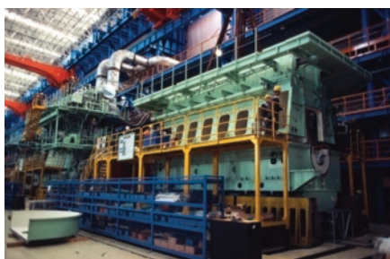
Figure 33.72 Built in Finland the Wärtsilä, RT-flex is the world's largest and most powerful diesel engine.
