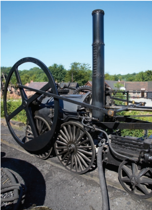
Figure 33.22 A rim type flywheel forming part of an early steam engine. This design gave a larger moment of inertia than for a solid disc design of the same mass as the mass is positioned further from the axis of rotation.
