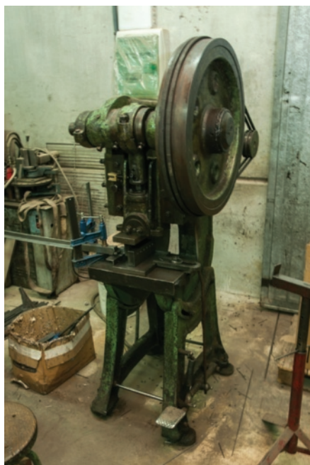
Figure 33.29 A metal press uses a flywheel to assist the motor.
