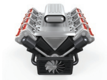
Figure 33.67 A V8 engine. Here you can see the two banks of four cylinders at an angle to each other.
