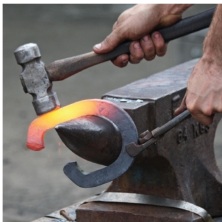
Figure 32.25 Blacksmiths can tell the temperature of the metal by observing its colour. Visible and infrared radiation are being emitted from the surface.
