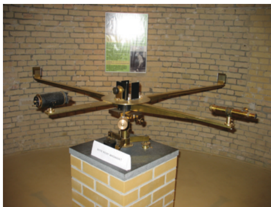
Figure 32.38 A Michelson–Morley interferometer. Although this apparatus is shown on a brick pillar, in the original experiment the interferometer took place in the basement of the laboratory. It was also placed on a heavy stone slab floating on a bath of mercury. This was to prevent any vibrations from affecting the measurements.
