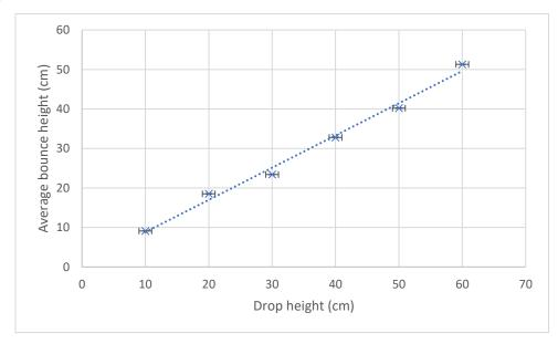
6 Using the value of the gradient calculated by Excel, the efficiency is 82 %. By drawing lines of steepest and shallowest fit, the uncertainty can be estimated at 3%.
