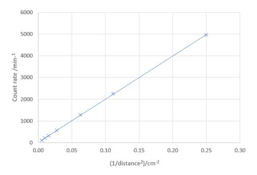
The graph is a straight line and Excel gives an intercept of 14. This suggests a background radiation level of 14 counts min<sup>-1</sup> which is a reasonable level, and the results therefore support the student's hypothesis.
