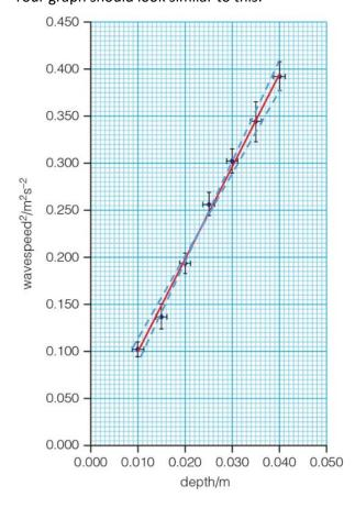
4 Using  $v = \sqrt{gd}$  to obtain  $v^2 = gd$ . Comparing to the equation of a straight-line, y = mx + c shows that the gradient of the graph will be equal to acceleration due to gravity.
