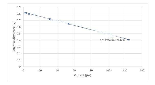
c) Comparing  $V = \varepsilon - Ir$  to  $y = mx + c \Rightarrow$  the gradient of this graph is -r and the intercept is  $\varepsilon$ . [1] From graph above,  $-r = -0.0033 \text{ V/}\mu\text{A}$
