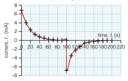
2 Total charge = area under charging or discharging portion of graph. Use a 'counting squares' technique to determine this value.  $Q_0 = 0.126 \text{ C}$
