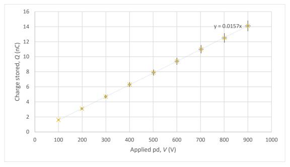
The maximum and minimum values of the gradient are dictated by the error bars. The maximum gradient is  $1.67 \times 10^{-7}$  Fm<sup>-2</sup>, and the minimum is  $1.47 \times 10^{-7}$  Fm<sup>-2</sup>. This gives an uncertainty in the gradient of  $\pm 0.10 \times 10^{-7}$  Fm<sup>-2</sup>.
