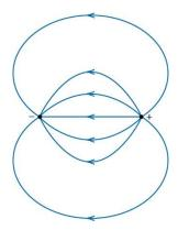
ii) The direction of the field at D is parallel to AB and directed to the left. [1]
