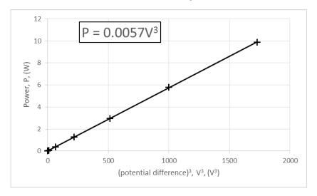
6  $P = V^2/R$ . The resistance of the rheostat is constant, hence P only varies with  $V^2$ . In the bulb, R increases with V, adding another term to the power equation in terms of V – this means  $P \propto V^3$  – from best-fit.
