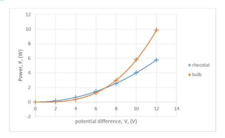
In both cases, P increases with V. The bulb increases in the form  $P = kV^3$  (using Excel to fit best-fit curve) and the rheostat increases in the form  $P = V^2/R$ . The rheostat initially has P increasing at a greater rate than for the bulb. At V = 5 V, both components have the same power. As V increases the power of the bulb increases at a higher rate than the rheostat.
