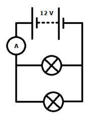
b) Current flowing through each bulb,  $I = \frac{P}{V} = \frac{32}{12} = 2.6 A$  [1]
