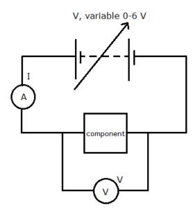
[1 mark for correct electrical circuit; 1 mark for suitable apparatus]
