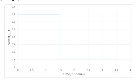
b) Total charge = area under graph =  $(0.70 \text{ A} \times (90 \times 60) \text{ s}) + (0.12 \text{ A} \times (120 \times 60) \text{ s})$ = 3780 + 864= 4644 C = 4600 C (2 sf)
