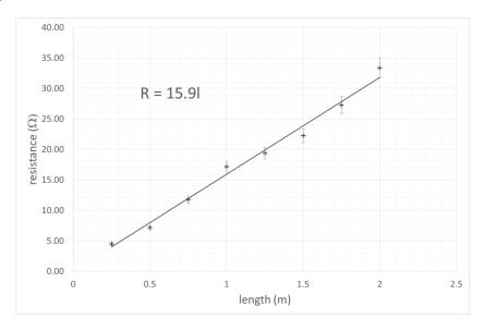
7 Excel should calculate the gradient to be 15.9  $\Omega$ m<sup>-1</sup>.
