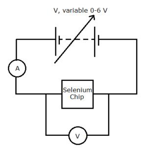
b) Temperature (kept constant) – digital thermometer situated close to chip; pd, V across selenium chip – digital voltmeter connected across the chip; current, *I* in circuit – digital ammeter/milliammeter connected in series with the chip; length, width and depth of chip, *I*, *w* and *d* – Vernier calliper (take 3 readings of each and average).
