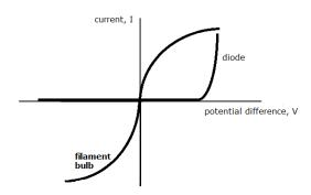
b) Resistance,  $R=\frac{V}{I}$ . As V increases, so does I, but proportionately less than the increase in V [1]. This indicates that the ratio  $R=\frac{V}{I}$  increases with V [1].
