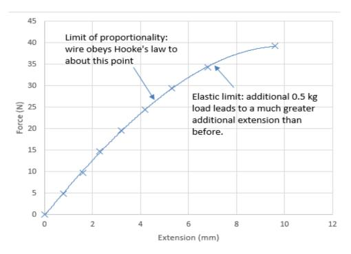
There is no indication in the sample results of when the wire breaks, but it may be at a load of 4.5 kg.
