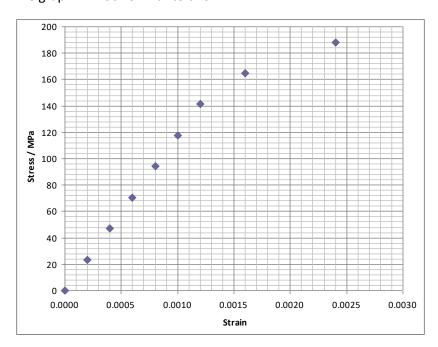
To calculate Young Modulus, you need to find the gradient of the straight line section of the graph (up to stress of approximately 140 MPa). The gradient of the graph should be approximately 116 GPa.
