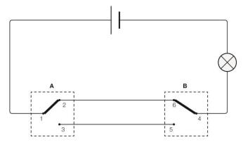
(Note that the bulb would also light if the switches were in positions 1 to 3 and 5 to 4.) (2 marks)
