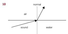
Sound bends towards from the normal because it is faster in water than in air.
