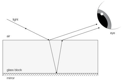
(Air/glass refracted ray for 1 mark, glass/mirror reflected ray for 1 mark, glass/air refracted ray for 1 mark)
