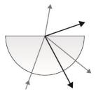
8 a) When the angle of incidence in plastic is 42°, the angle of refraction at the plastic/air boundary (1 mark) is 90°. (1 mark)
