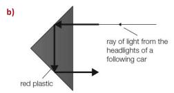
(1 mark for extending incident ray to far plastic edge without changing direction, 1 mark for correct first reflection with angle of incidence/reflection of 45°, 1 mark for correct second reflection with angle of incidence/reflection of 45°, 1 mark for crossing final plastic/air boundary without changing direction)
