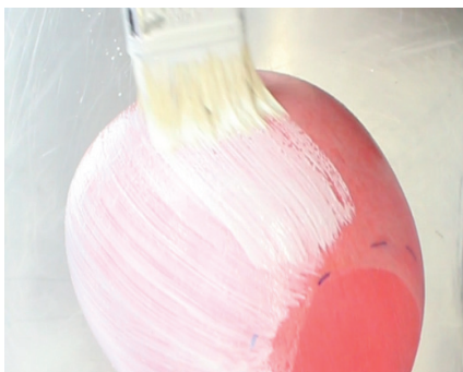
Step 6 – Apply the next layer, ensuring full coverage and check that the edges remain thin.
