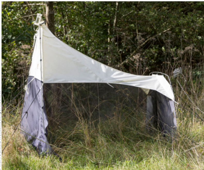
Figure 3 Stages of the BIOSCAN process for DNA barcoding insect biodiversity. (a) A malaise trap used to collect monthly samples for BIOSCAN. The pot of ethanol where samples collect is visible on the top left of the trap. (b) A 96-well plate showing separation of insects into individual wells for DNA extraction and PCR. (c) Massively parallel sequencing of DNA barcodes on a PacBio machine
